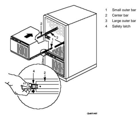
Figure 7. Installing the Server in the Rack
